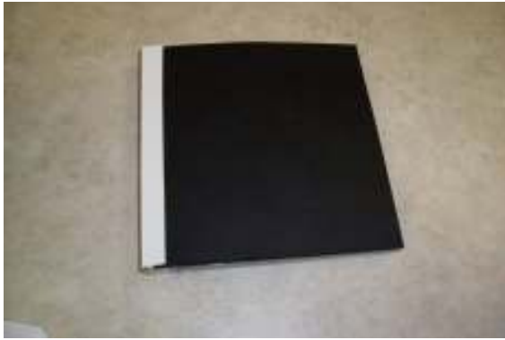
Finished book block. Heavy weight cover stock trimmed off before casing in.
