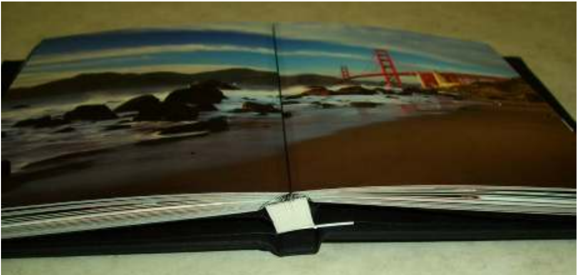
Heavy cover stock applied during perfect binding keeps the spine of the book block rigid
