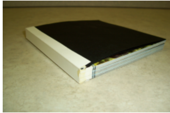
Finished book block. Heavy weight cover stock trimmed off before casing in.
